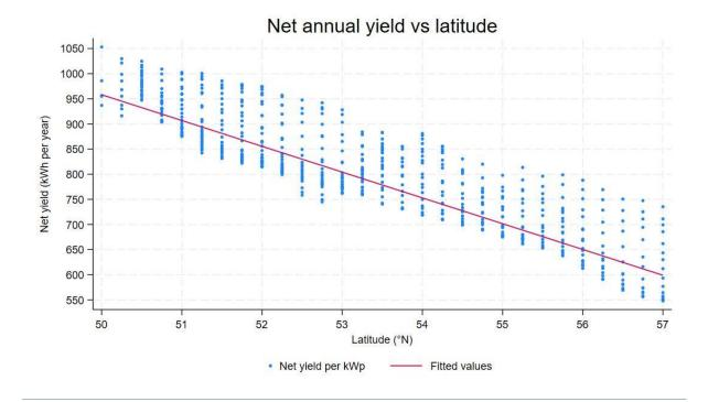
The fitted line indicates that the expected value of annual net yield from solar panels will decrease by about 50 kWh per kWp of peak capacity for each degree of latitude north of 50°N. At an average price of about £72 per MWh in 2024 that translates to £3,600 per year per MWp. For a solar farm with a capacity of 100 MWp that is a difference in gross revenue of £1.8 million per year between locations in Somerset, Hampshire or Sussex at a latitude of 51°N or in the Lothians at a latitude of 56°N.
